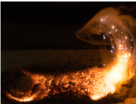
Self propagating exothermic reaction of hot topping powder
